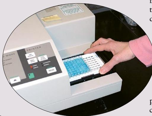
**ELISA TEST: The enzyme-linked immunosorbent assay, or ELISA, test is particularly sensitive to high-potency medications, can be conducted rapidly, and can be read by the eye.**
