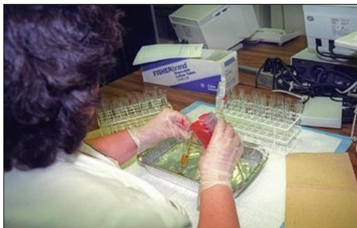
**PREP WORK:** An analyst pours a portion of each urine sample into test tubes. These sub-samples, called aliquots, are delivered to the thin-layer chromatography and ELISA testing areas.
